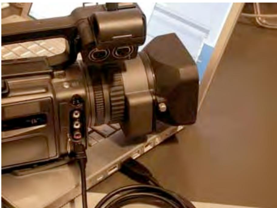
Figure 3: *FireWire* enables digital video data to be transferred directly from a camcorder to a computer for editing
