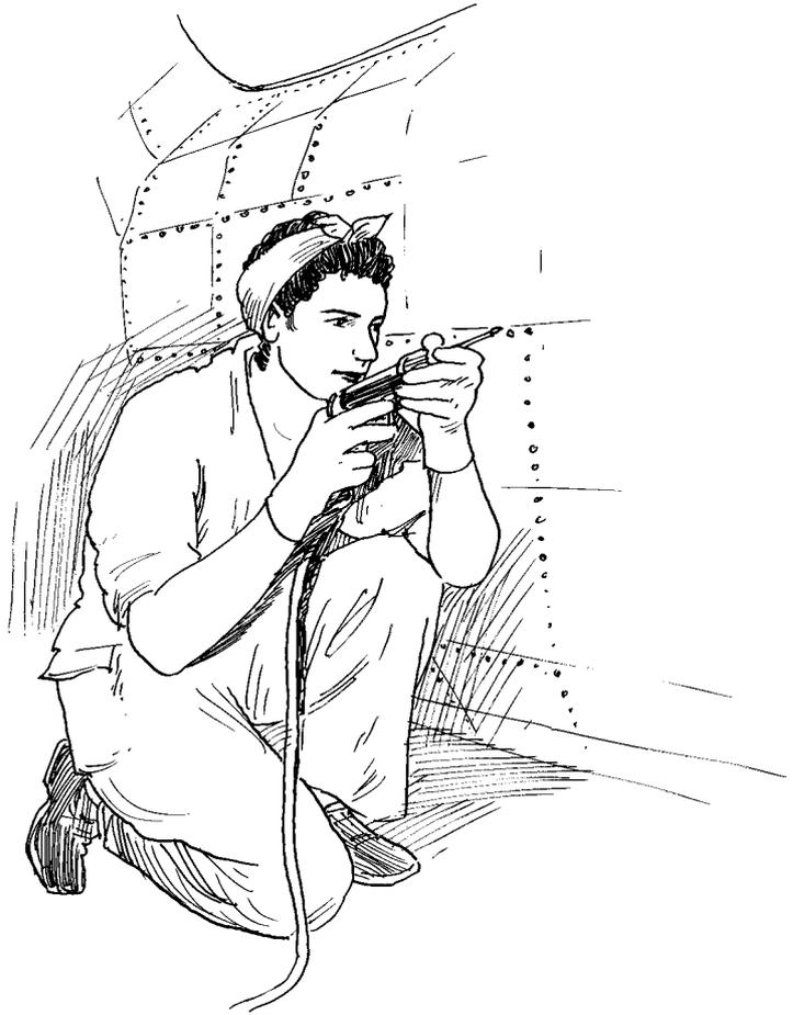
Rosemary rivets (attaches) a large sheet of metal onto a war plane.
